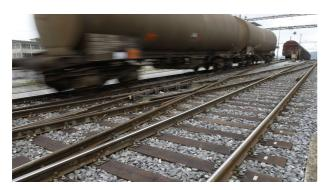
In the case of derailment wooden sleepers don't break despite being struck by metal wheels. If a derailment occurs the track width remains the same and the track system thus remains open to traffic. This is not the case for concrete and metal sleepers; concrete sleepers break and steel sleepers bend.
